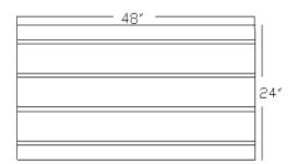
Master Panels, 10 pcs., 24" x 48" PLEASE NOTE: Panel System for <sup>3</sup>/<sub>8</sub>" tubing is <sup>3</sup>/<sub>4</sub>" thick. Panel System for <sup>1</sup>/<sub>2</sub>" tubing is 1" thick.
