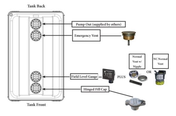
**Note:** Some installations may require a normally closed normal vent vs. an open vent cap. This vent opens when the tank is being filled to avoid tank pressurization and also opens when the tank contents are being pumped out to avoid vacuum accumulation. Otherwise it is closed, preventing infiltration of contamination from outside the tank and evaporation of the tank contents.
