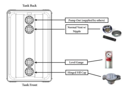
All accessories are supplied with 2 inch MPT threads and install directly on the Roth Metallic NPT adapters.
