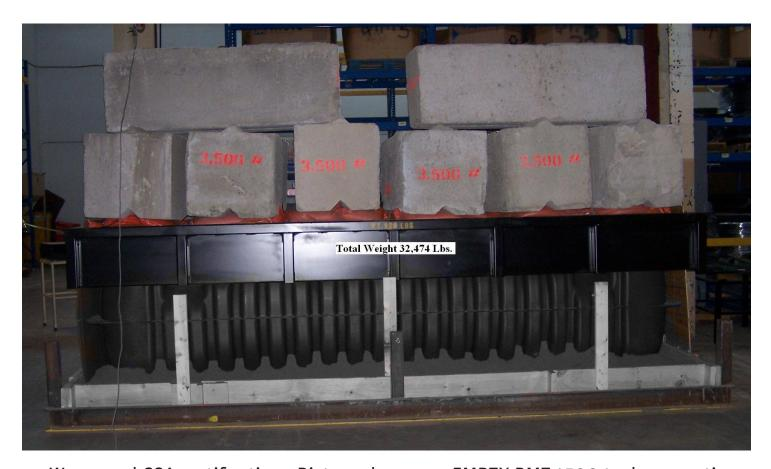
We earned CSA certification. Picture shows our EMPTY RMT-1500 tank supporting 32,474 lbs. of concrete. This test went on for 3 days. August 2007
