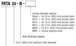
Fiberglass riser tank adapter
