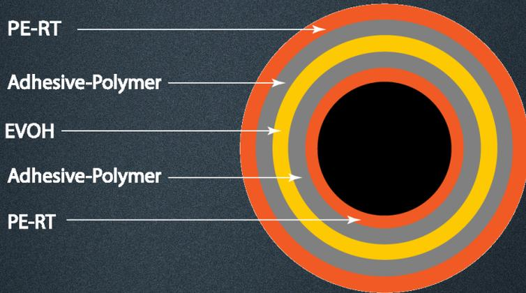
The five-layer pipe consists of a layer of ethylene vinyl alcohol polymer (EVOH) sandwiched between two layers of Polyethylene Copolymer Resin and two layers of adhesive. This structure provides the outstanding long-term hydrostatic design strength demanded by hydronic heating applications.
